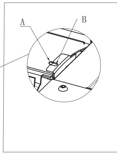
Adjust solution if hole "A" and hole „B“ are not concentric.
