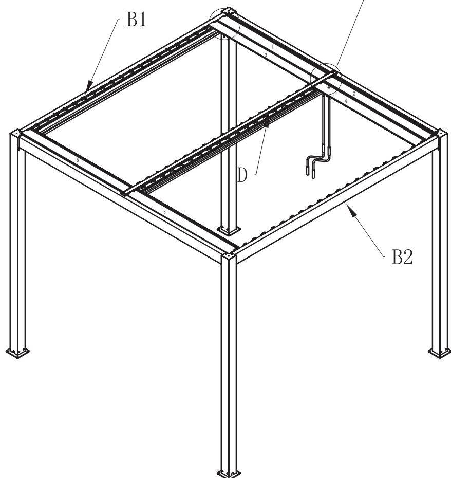
First, fix screw K2 with gasket K3 align with hole below the beam D, then same to beam C. Insert the other flap in turn.
