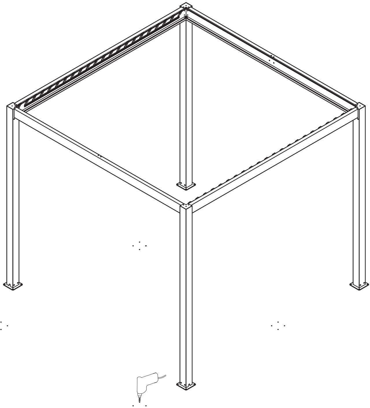
Place the plastic expansion pipe in the bottom hole of the column. Then move the product back to the hole drilled, align holes of the column bottom plates with the hole drilled on the ground. Then set L1 into the woodworking screw L, and fix it with the ground separately.
