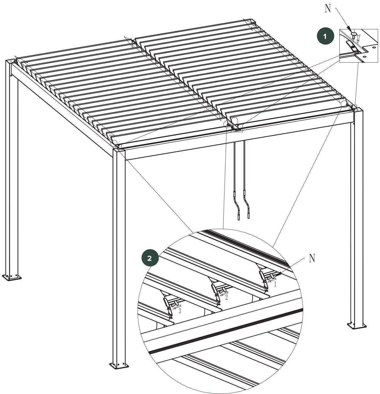
Turn on the flap to half position, insert the plastic jam N into hole of two ends of each flap in turn.
