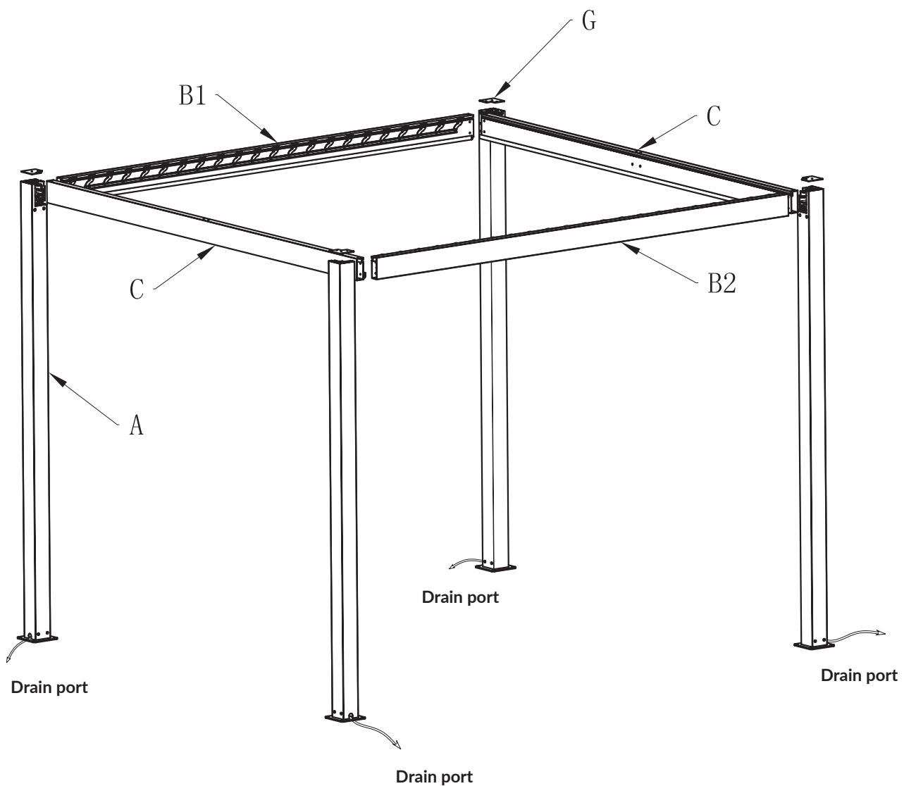
The two ends of one front and rear beam C are respectively placed on the corner connectors on the column, and the screws K1 are tightened.
