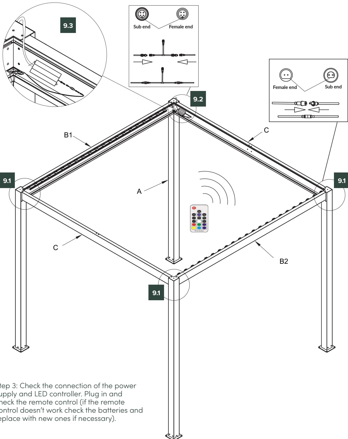
Step 3: Check the connection of the power supply and LED controller. Plug in and check the remote control (if the remote control doesn't work check the batteries and replace with new ones if necessary).
